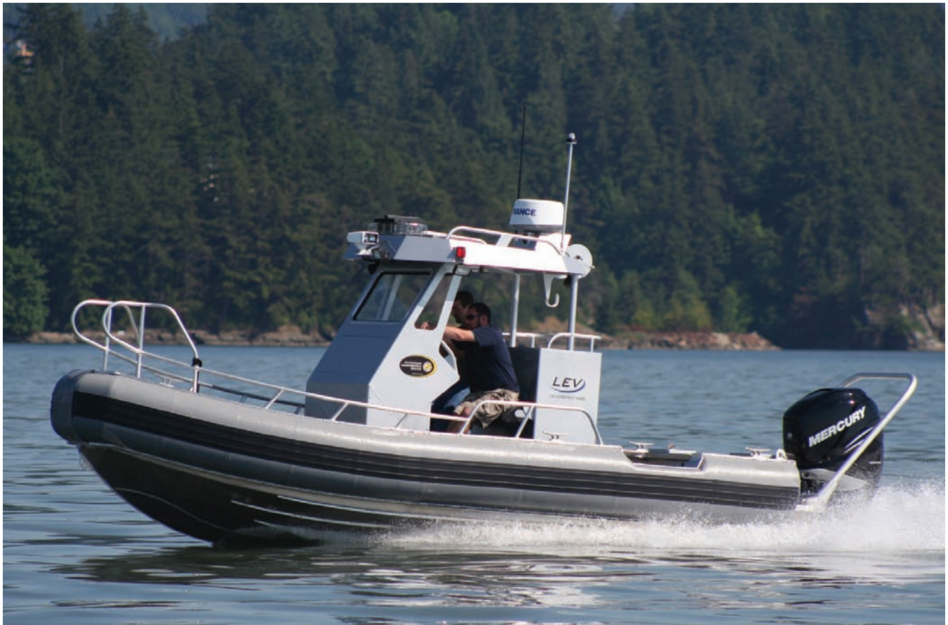
ACB's 21-ft Law Enforcement Vessel (LEV). Available with an air or foam hybrid collar for fendering and additional flotation, the LEV was designed by marine patrol officers specifically for maritime law enforcement. (Photos courtesy Aluminum Chamber Boats)
