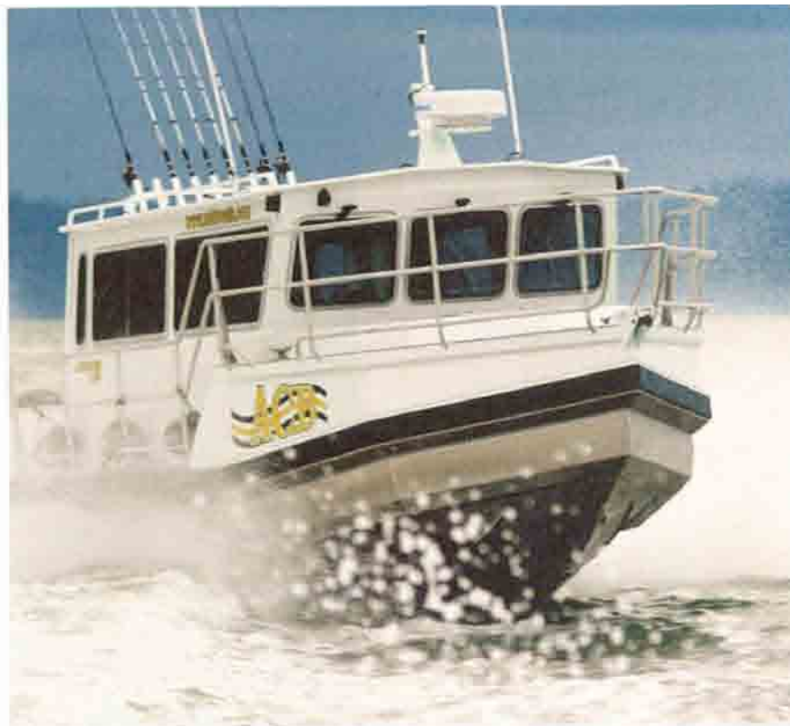
Boats with flotation collars are ideal for Alaskan waters—not only are they safer, but they also provide a drier and softer ride.
